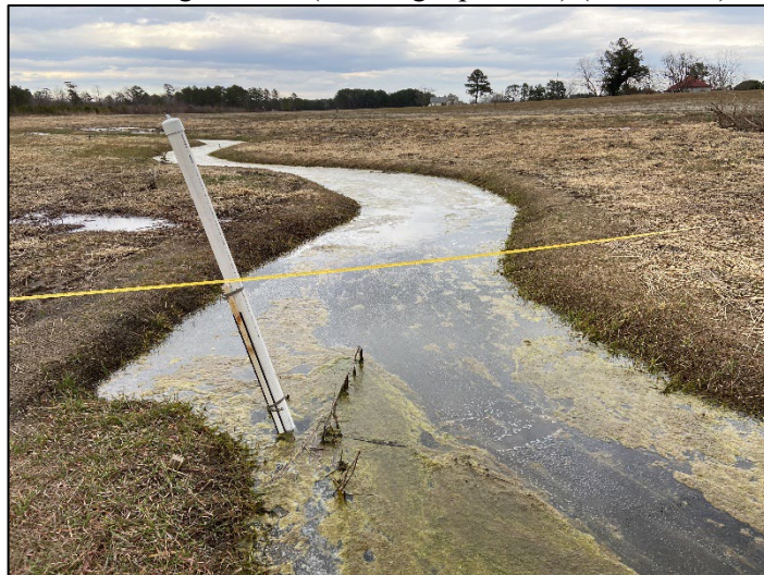
Stage Recorder JH1-B (Looking Upstream) (2/16/2022)
