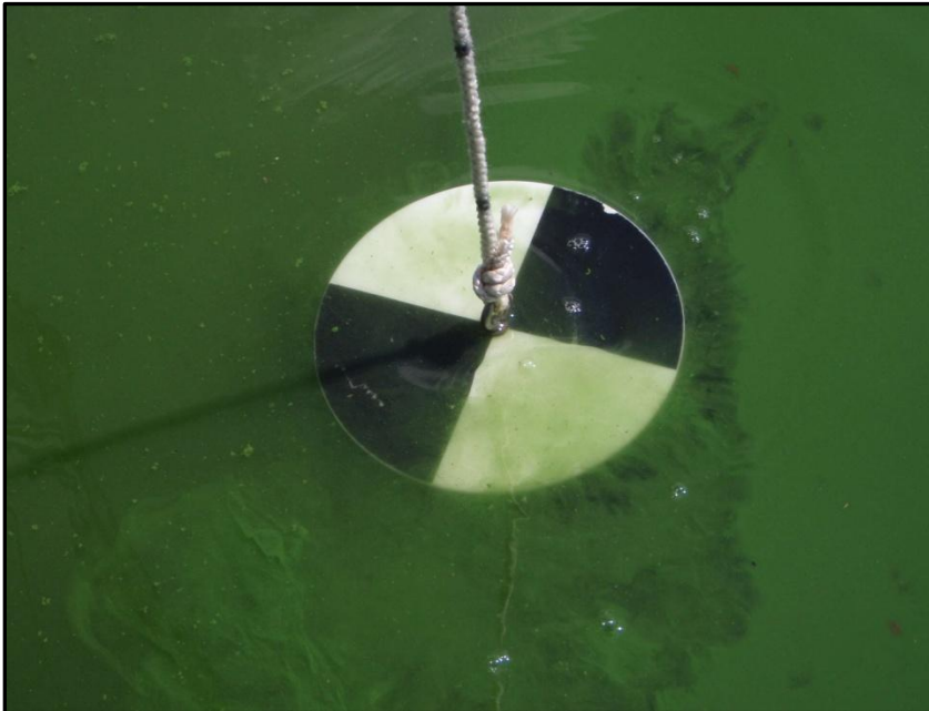
Figure 6. Secchi disk at the surface of Lake Tabor during the August 7, 2011 algae bloom.
