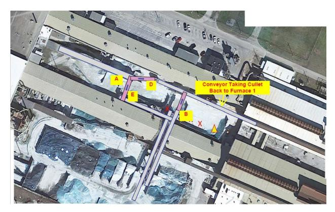
The mitigation project will reduce the usage of a front-end loader transferring the cullet in the middle yard by over 80%. The project will reduce total fugitive PM emissions by 92% (from 2.28 tons/year to 0.17 tons/year).
