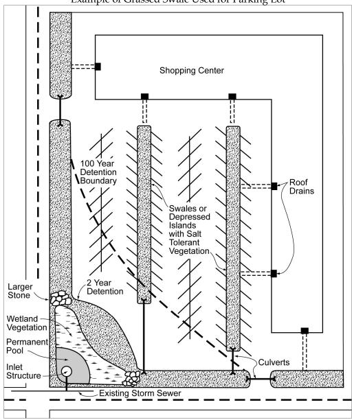
**Figure 14-3** Example of Grassed Swale Used for Parking Lot
