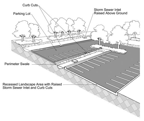
**Figure 14-5** Parking Lot Swale Drainage (from NIPC, 1993).
