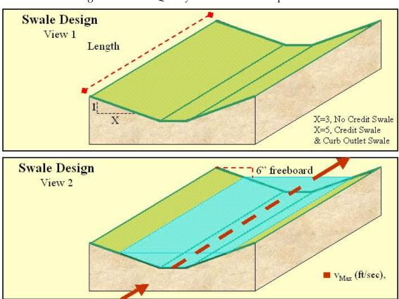
**Figure 14-6** Diagram of Water Quality Grassed Swale Requirements
