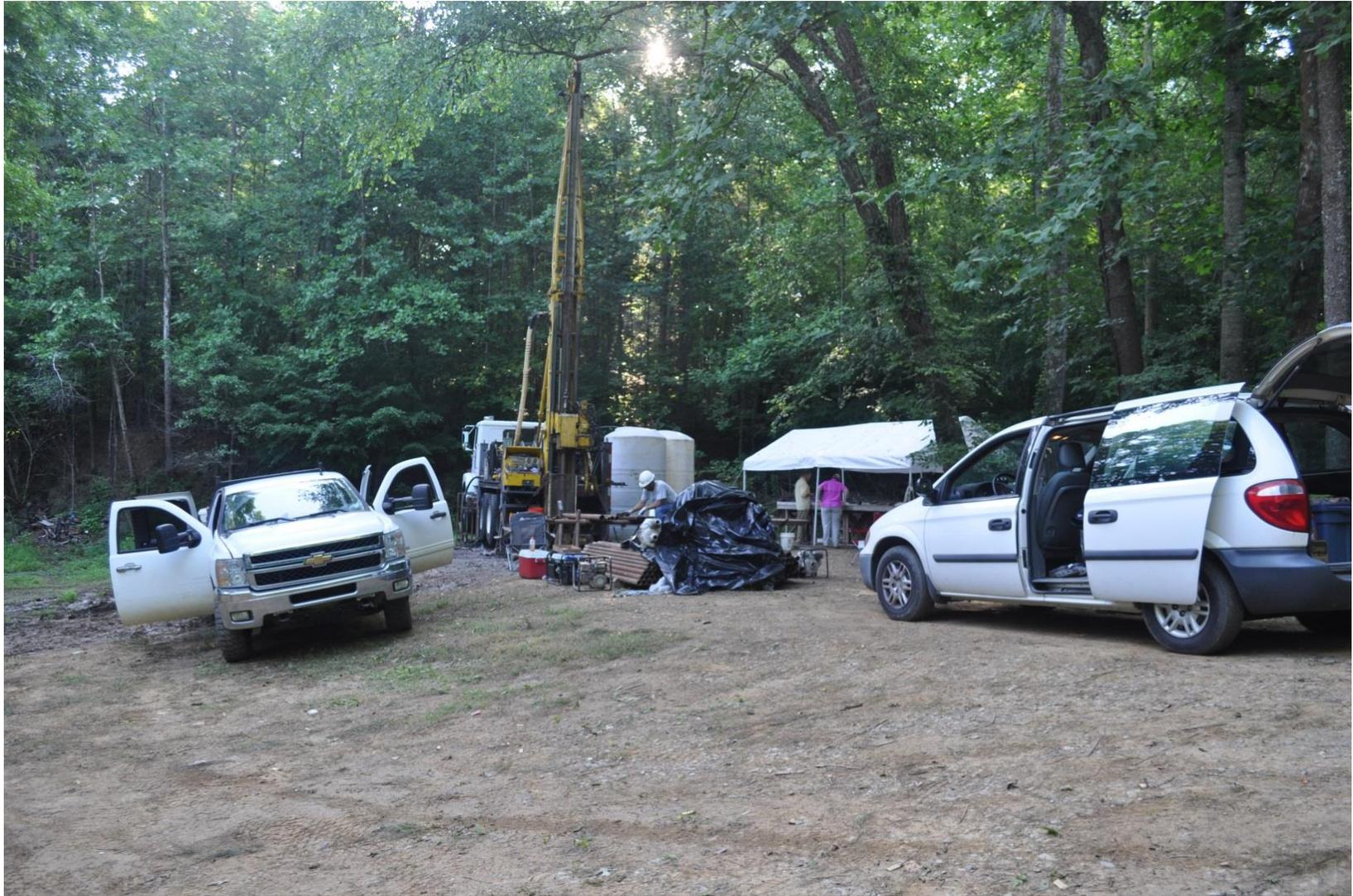
**Fig. 1.** Wire line core drill used for the Town of Walnut Cove (SO-C-1-15) stratigraphic core hole. The drill rig is a truck mounted Christianson CT-14 core drill. Visible in the photograph are support vehicles, some of the drill rods, cement (covered with black plastic), and logging table (under white tent).
