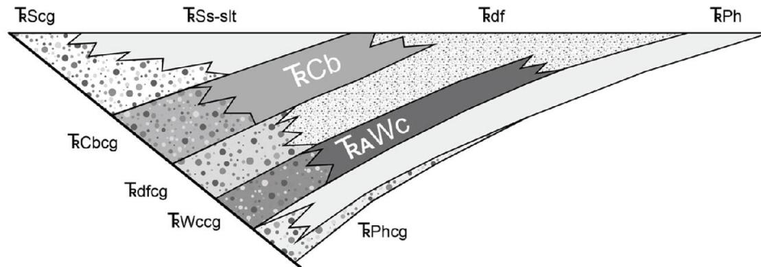
**Fig. 7.** Cross section across the Dan River basin (from Olsen and others, 2015). The cross section corresponds to a line approximately parallel to U.S. Highway 220 in Rockingham County, North Carolina from the eastern basin margin to the basin’s western margin. A thin coal and carbonaceous interval is present in North Carolina but not in the Virginia portion of the basin.
