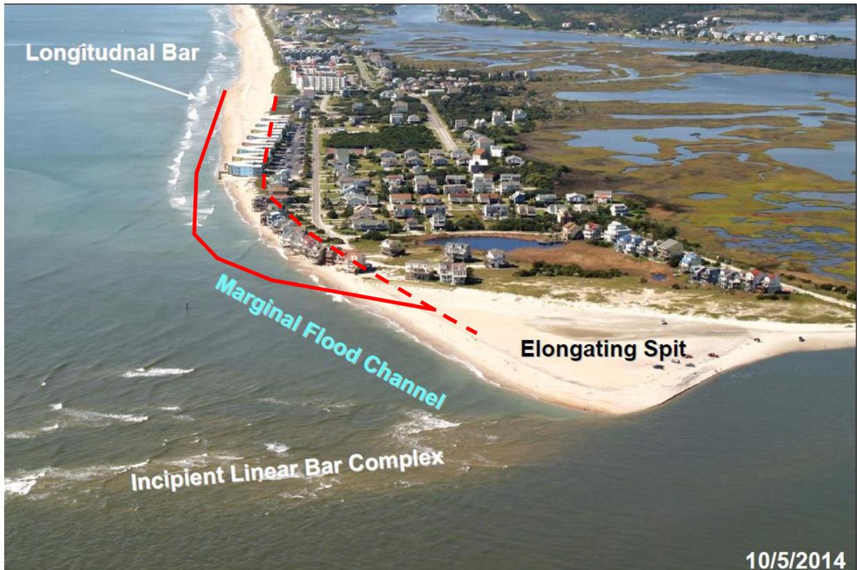
**Figure 10. Schematic showing post-construction shoreline orientation (solid red line) and natural shoreline (dashed red line).**
