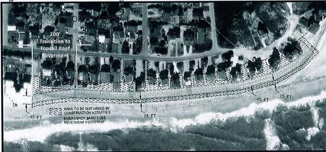
Figure B. Plan view of sand bag revetment footprint, proposed area to be disturbed, transition to Topsail Reef revetment and location of the First Line of Stable Natural Vegetation (FLSNV).
