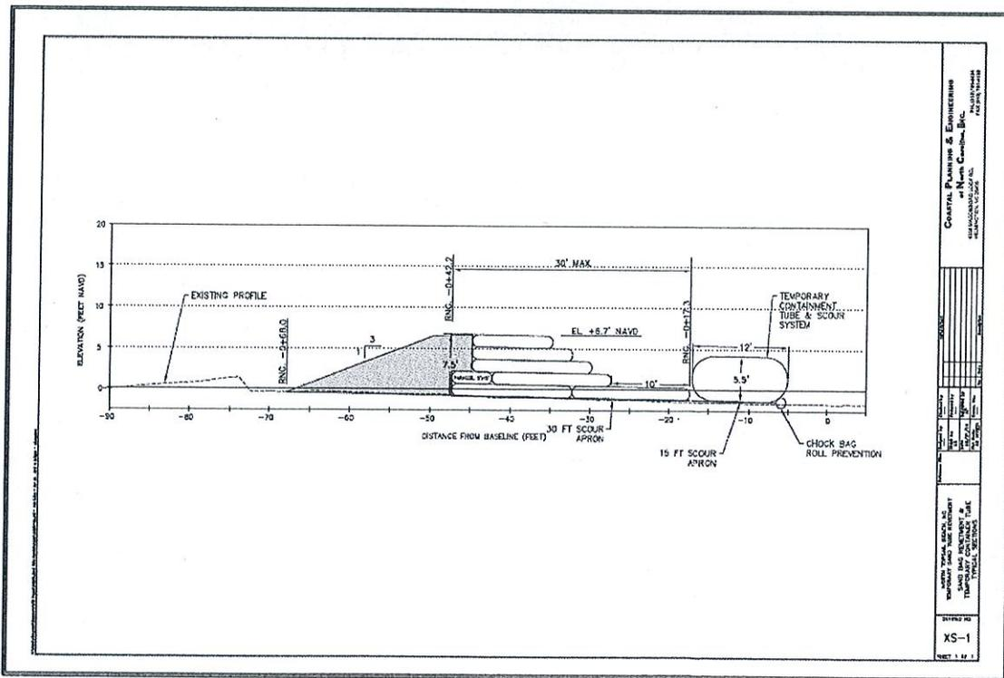
Figure 1. Typical cross-section of sandbag revetment and temporary containment tube.
