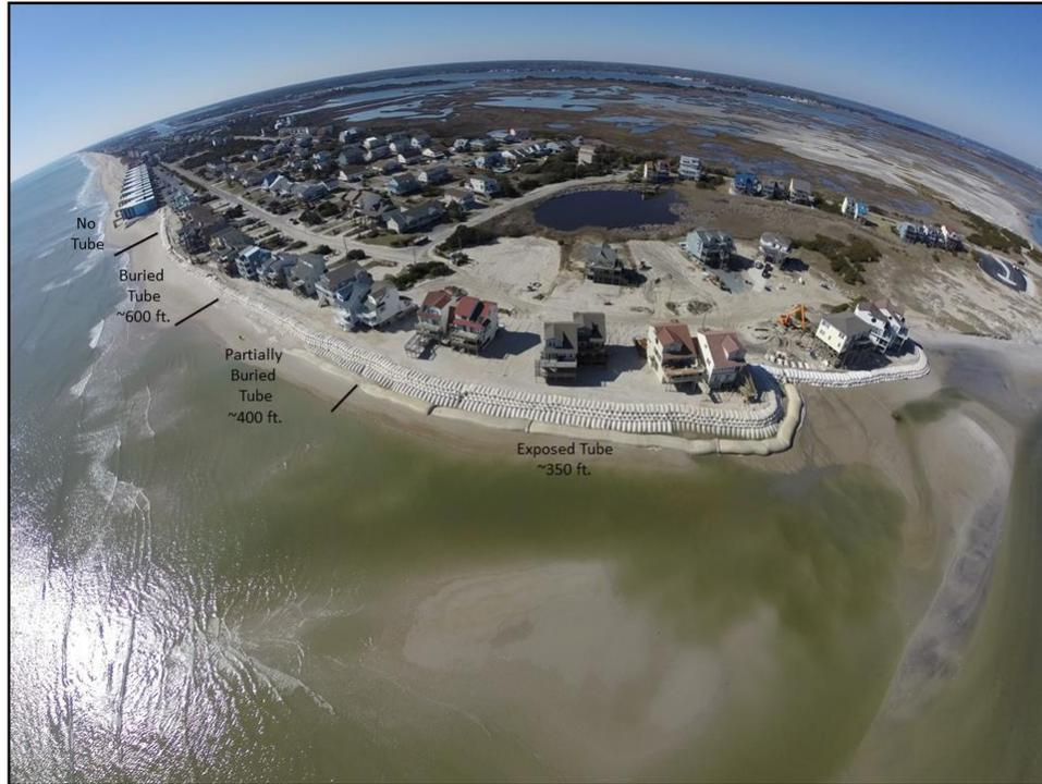
**Figure 2. March 20, 2015 drone aerial photo of sandbag revetment.**
