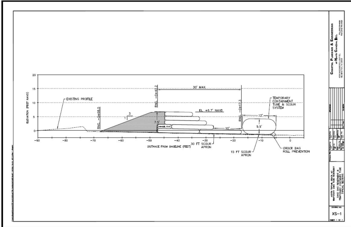
Figure 1 – Cross-Section of sandbag revetment and temporary containment tube.
