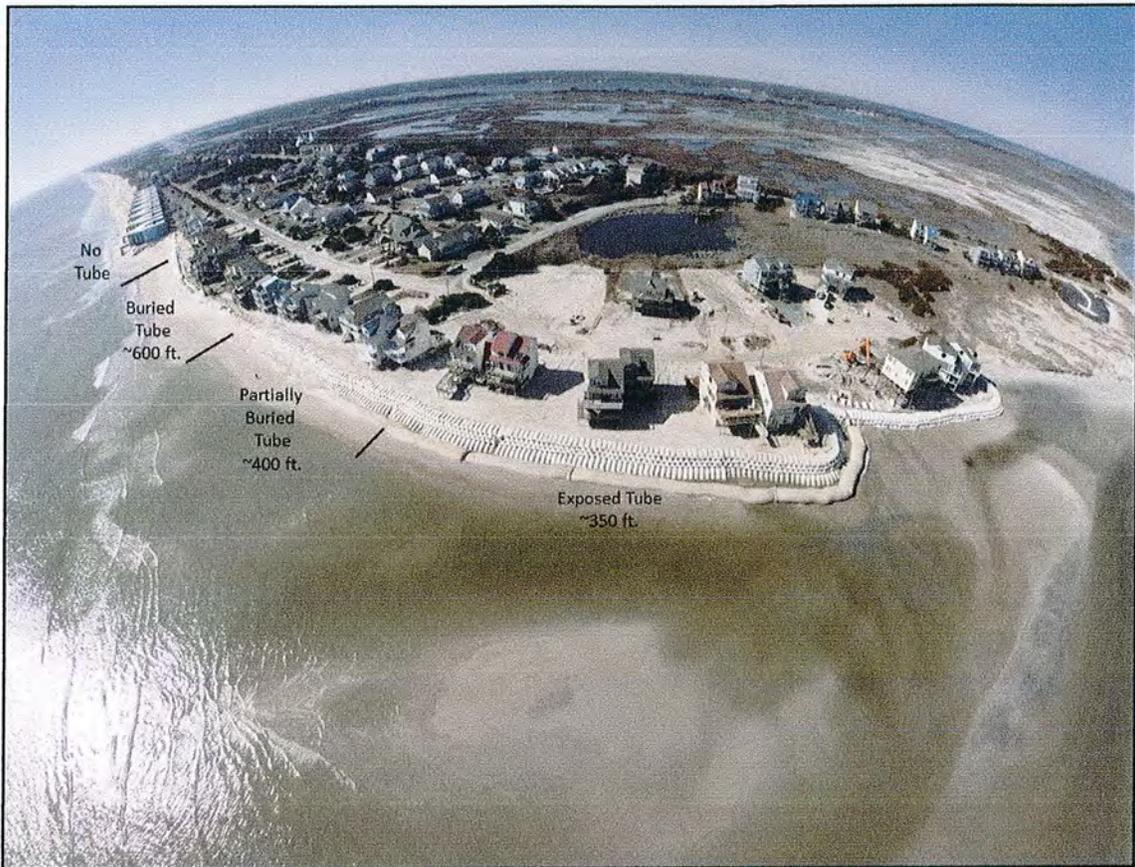
**Figure 1. Aerial photo of the sand bag revetment project area taken February 20, 2015 showing the condition of the tube. (Photo Courtesy of Mike Capuano)**
