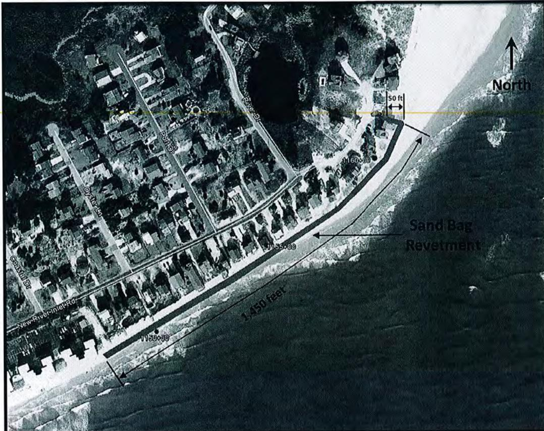
Figure A. Plan view of sand bag revetment
