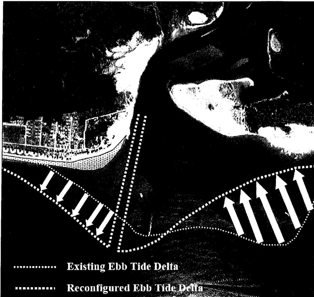
Figure 4. Schematic diagram showing the intended reconfiguration of the ebb tide delta as a result of the channel realignment project (Photo from October 2003).
