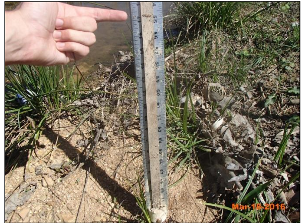
R Reach 3 Crest Gauge
