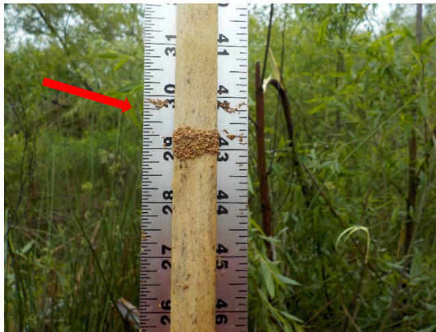
Crest Gauge @ Reach 2 – 30 in. (2.5 ft.)
