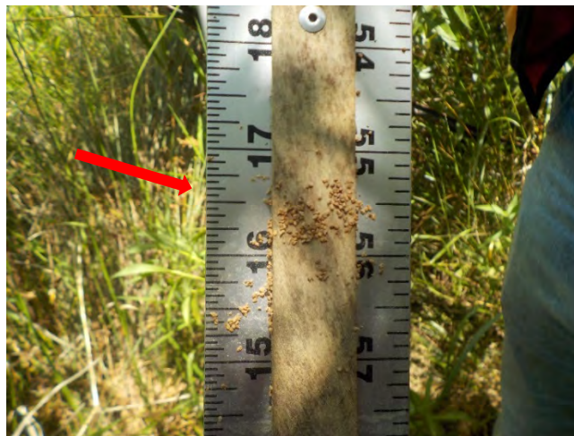
Crest Gauge @ Reach 3 – 16.75 in. (1.4 ft.)
