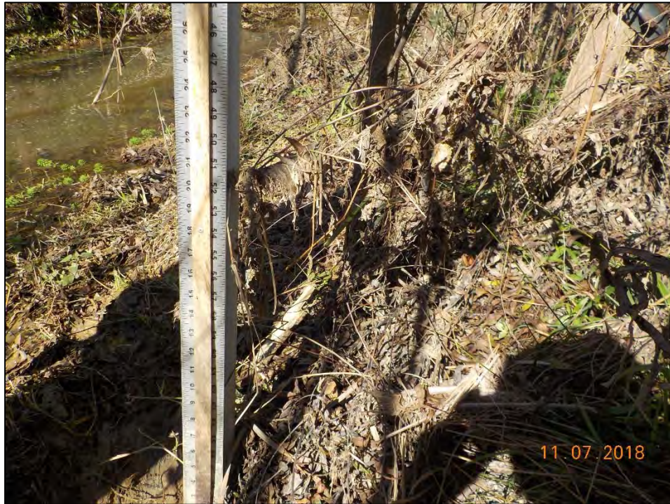
Wrack lines @ Crest Gauge Reach 2 – 0.66 feet
