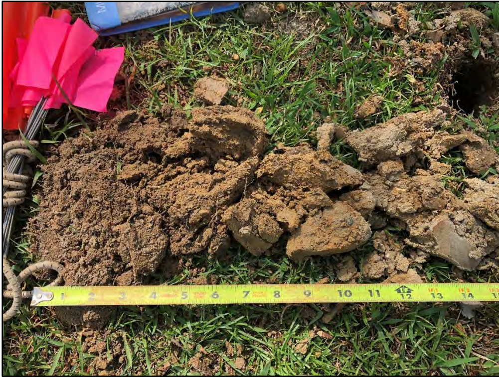
3. Hydric soil below toe of slope and edge of floodplain with A11-Depleted Below Dark Surface indicator at Profile # 117.
