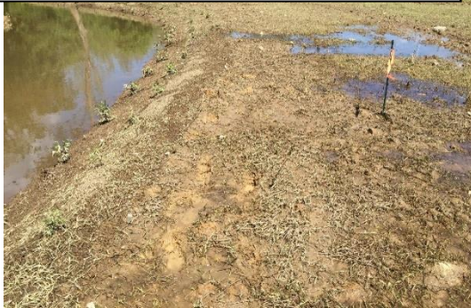
Bankfull Photo 1: Wrack, laid-back vegetation, and sediment in the floodplain of Travis Creek
