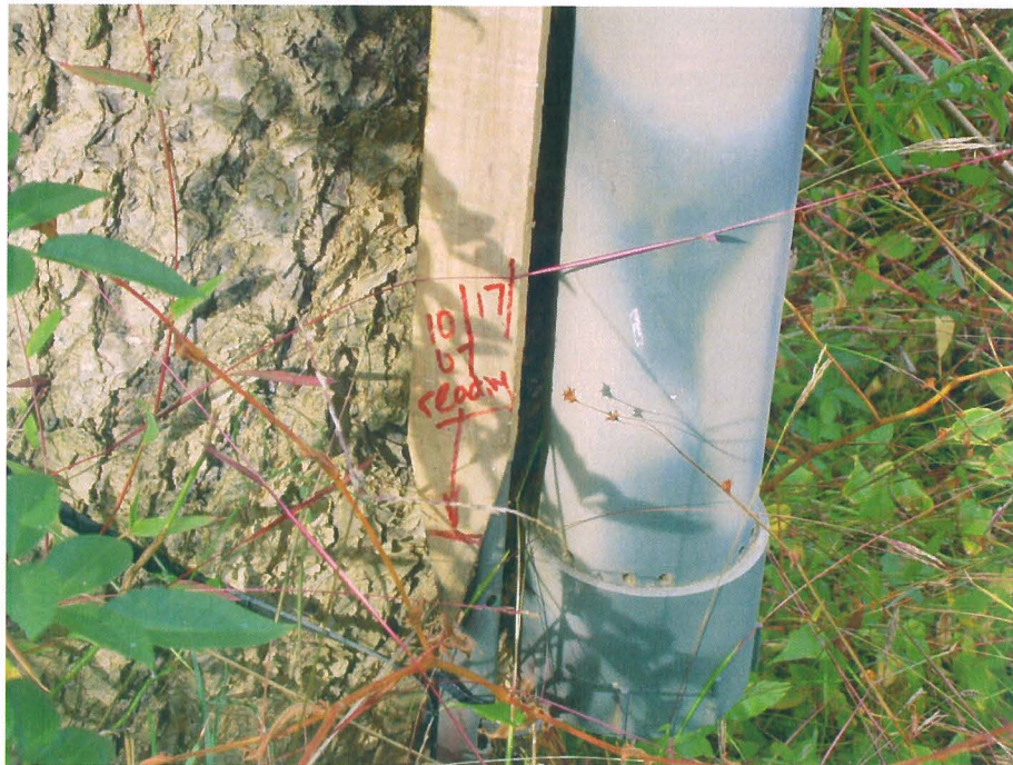
BF 2 Crest Gage 4 on Lower Bailey. (EMH&T, Inc. 10/17/07)
