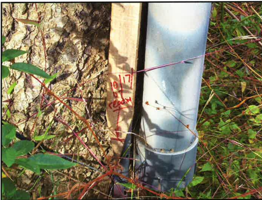
BF 2 Crest Gage 4 on Lower Bailey. (EMH&T, Inc. 10/17/07)
