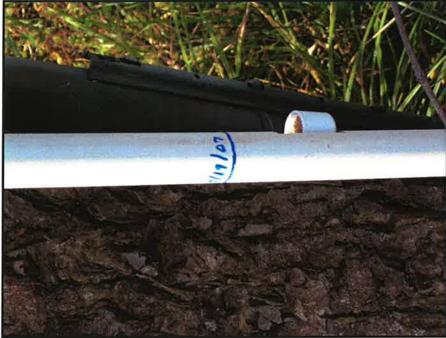
BF 1 Crest Gage 1 on UT1. (EMH&T, Inc. 7/19/07)
