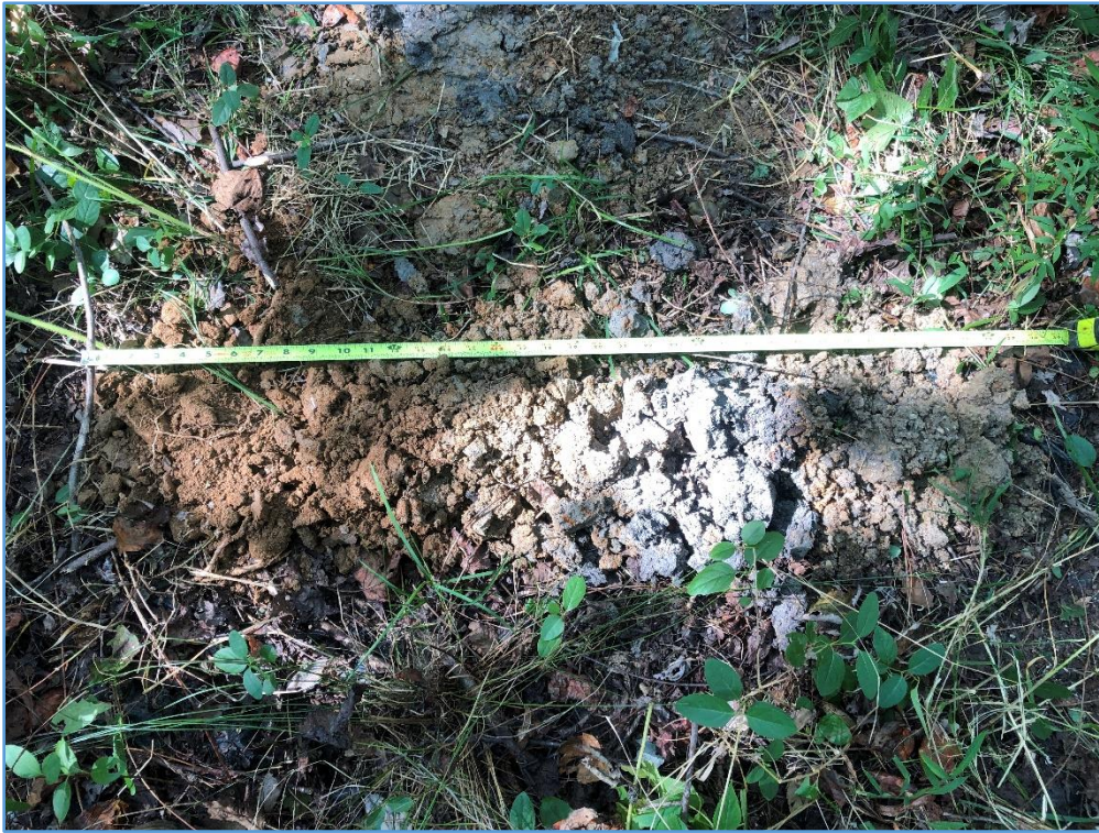
1. W4 Wetland profile. Meets the F3-Depleted Matrix and F8-Redox Depression indicators. SB#209.
