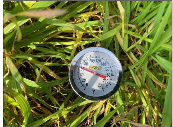
Soil temperature reading at 20 inches on 2/23/2023
