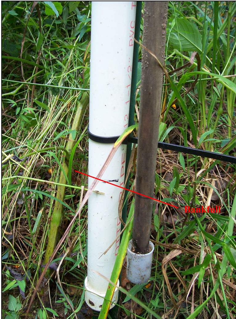
Photo 7. Crest gauge showing particulate deposited 6-8 inches above bankfull during a storm event in July 2007.
