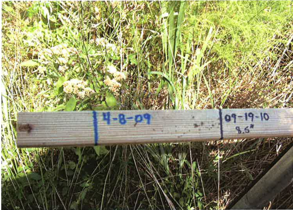
BF 1 Crest gage at 5+50 on UT1. (EMH&T, Inc. 9/19/10)
