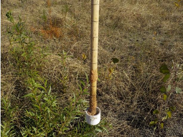
Crest Gauge 1 Reading 0.5' (10/8/2016)
