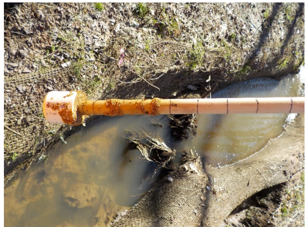
Crest Gauge 4 Reading 0.45' (2/3/2016)
