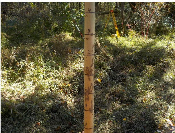
Crest Gauge 5 Reading 1.1' (10/8/2016)
