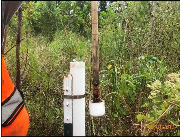
Crest Gauge 1 Reading 0.14'
