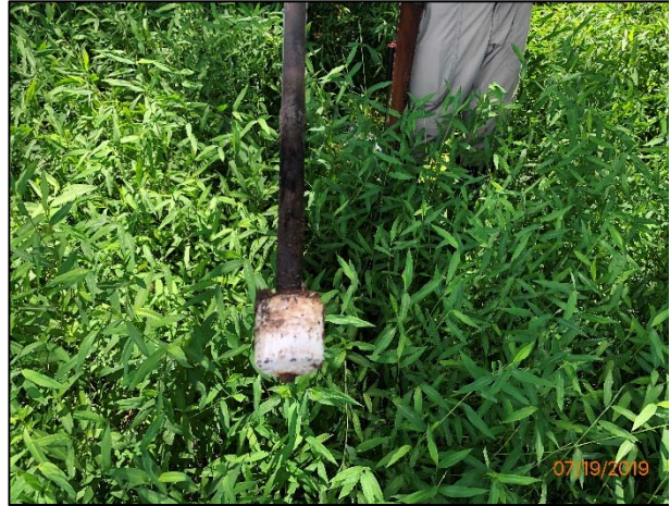
Crest Gauge 5 Reading 0.5'
