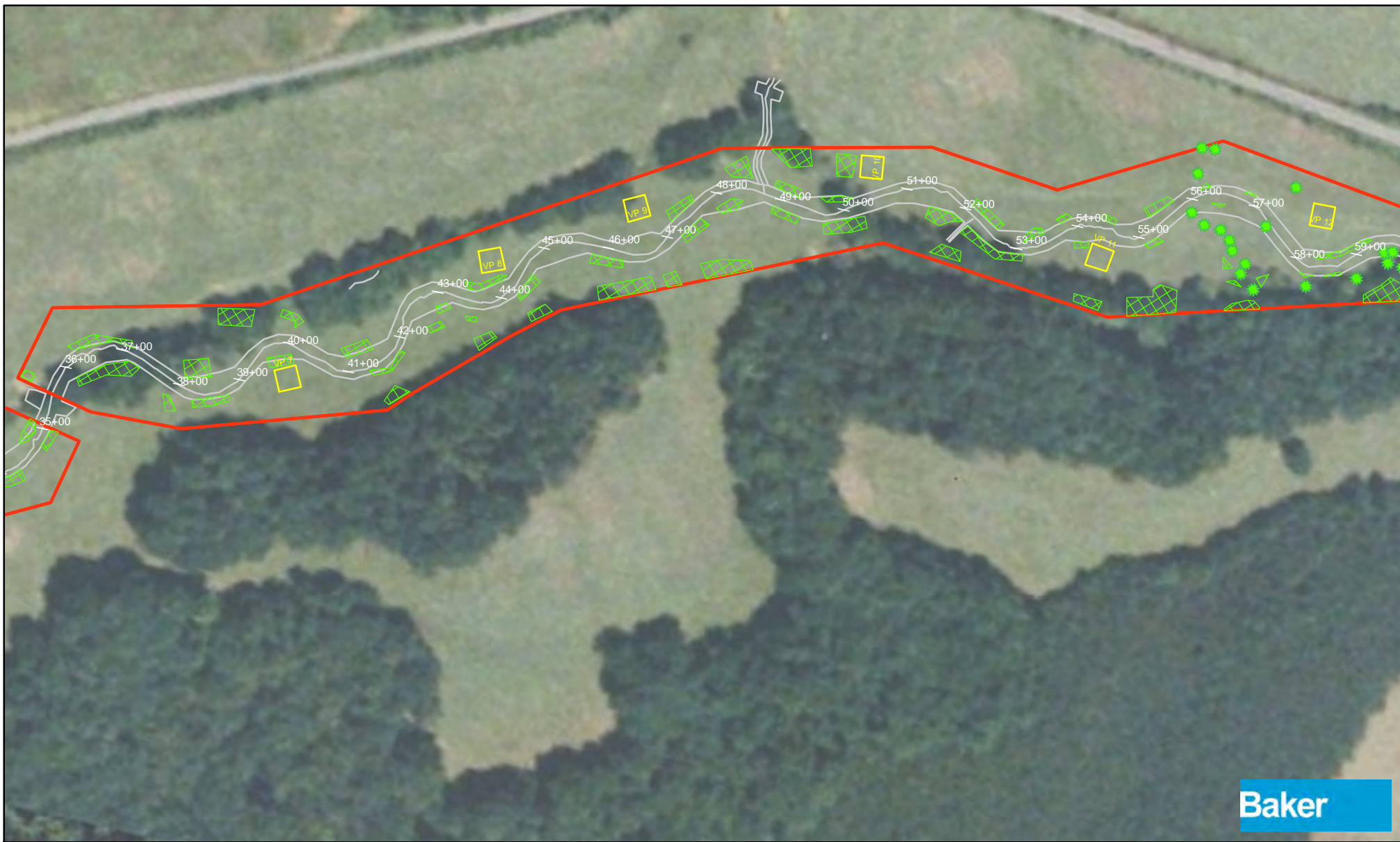
Figure C2: Vegetation Problem Areas BCC (Station 37+00 to 59+00)
