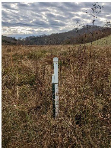
Crest Gauge 1. Reach 1 (Photo taken November 22, 2022)
