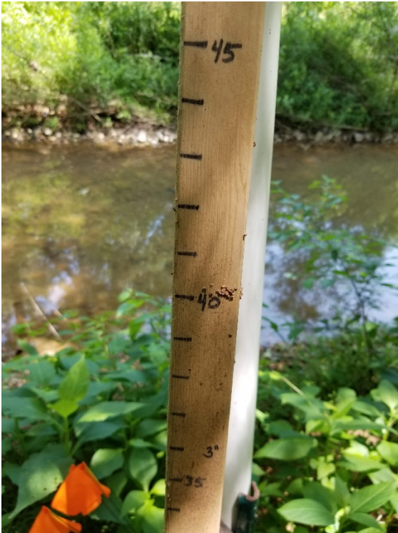
6/4/2019. Cork indicating stream flow reached 16" above bankfull flow (bankfull is at 24").
