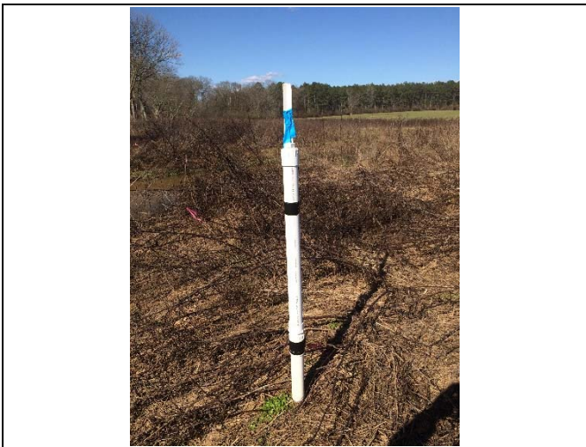
Reach HC-R2 – Crest Gauge at Station 31+75
