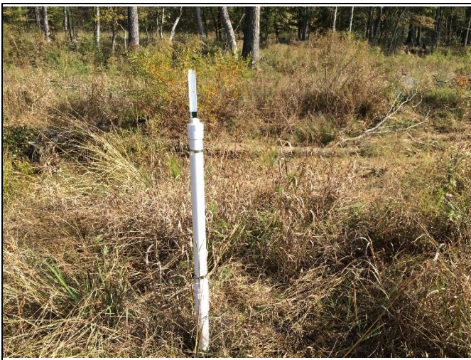
Reach UT4-R2 – Crest Gauge at Station 34+85
