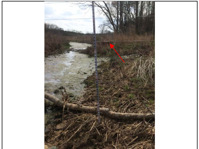
Reach HC-R1: Evidence of overbank flooding (debris caught in wires at cattle crossing ~3.3' height).
