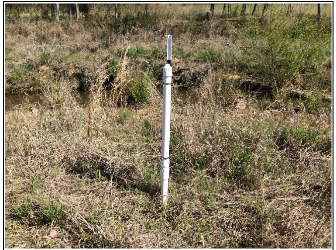
Reach UT4-R2: Crest Gauge at Station 34+85
