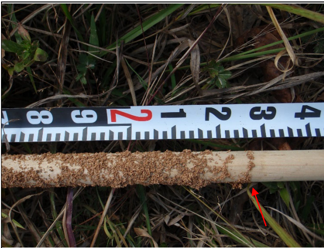
Reach UT4-R2: Overbank event of 2.26' (from Hurricane Florence on Sept. 15-17, 2018)
