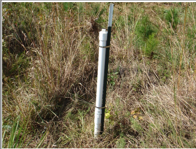
Reach UT4-R2: Crest gauge at Station 34+90
