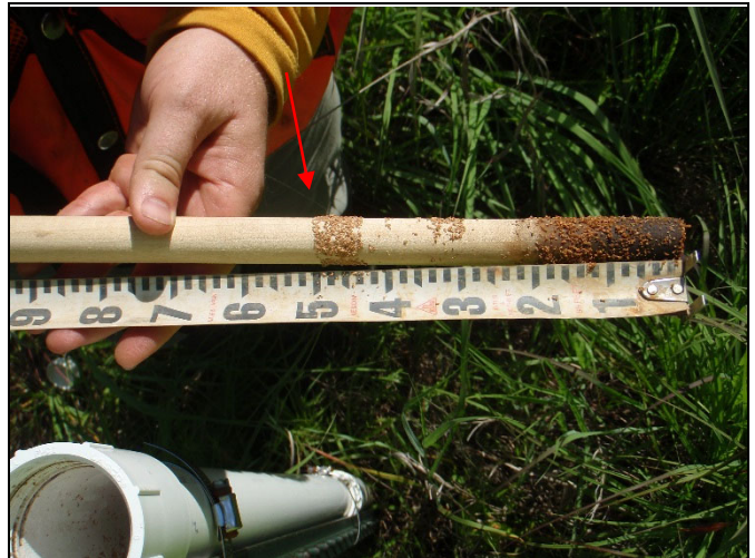
Reach UT4-R2 Crest Gauge: Overbank event of 0.50 ft recorded from 6/3/2018
