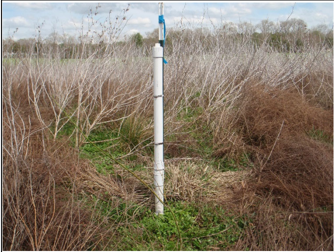
Reach HC-R2: Crest Gauge at Station 31+75
