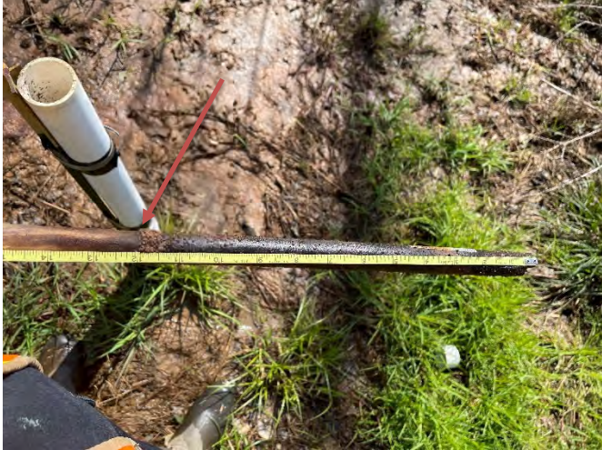
Manual Crest Gauge – Reading 3/16/23 (1.00')
