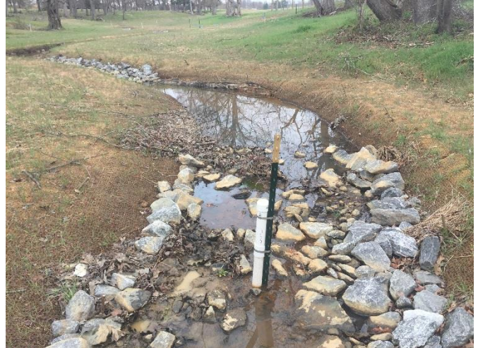
Automated Flow Gauge 1 – Reach 4
