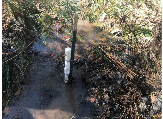
Automated Flow Gauge 1 – Reach 4
