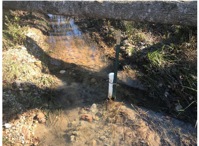
Automated Flow Gauge 3 – Reach T1
