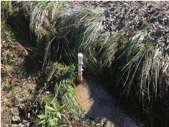
Automated Flow Gauge 2 – Reach T3
