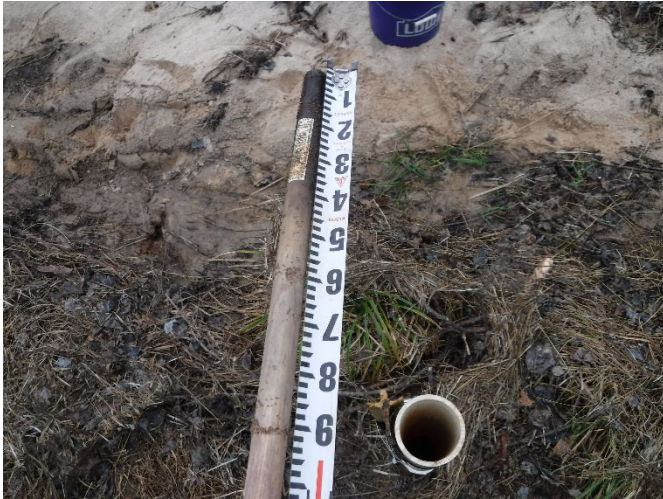
Manual Crest Gauge – Reading 1/24/2020 (.91')
