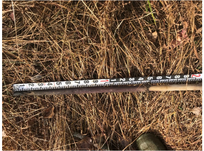
Manual Crest Gauge – Reading 11/6/2020 (1.49')
