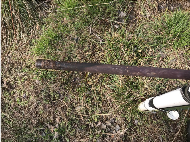
Manual Crest Gauge – Reading 3/22/22 (No Reading)
