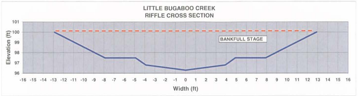
FIGURE 12 Typical Cross-Sections of New Channel
