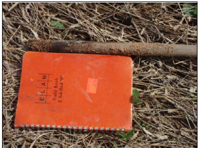
M3 crest gauge STA 55+50, April 8, 2014. Crest gauge reading of 0.82 feet.
