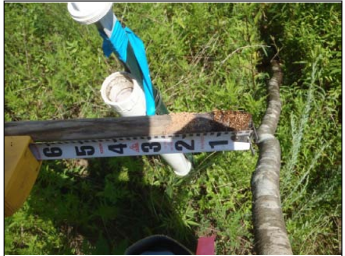
M3 crest gauge STA 55+50, July, 23 2014. Crest gauge reading of 0.23 feet
