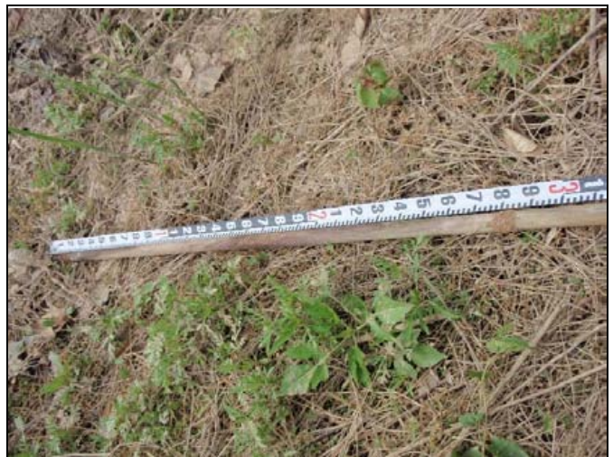
M3 crest gauge STA 55+50, April 30, 2015. Crest gauge reading of 2.85 feet.
