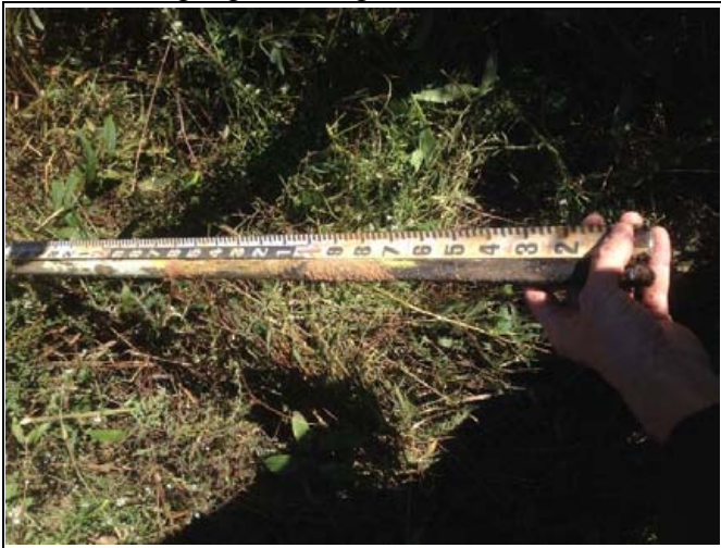
M3 crest gauge STA 55+50, October 19, 2015. Crest gauge reading of 1.60 feet.
