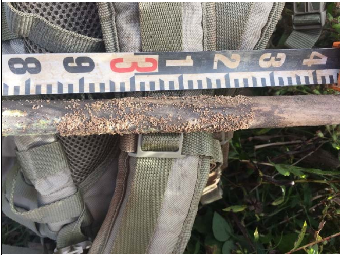
M3 crest gauge STA 55+50, October 11, 2016. Crest gauge reading of 3.24 feet.
