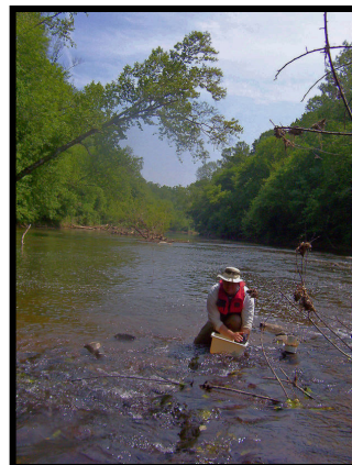
Photos 21 and 22. Sweep net and rock wash sampling for benthic macroinvertebrates at a reference station Source: EcoScience Corporation 2005
