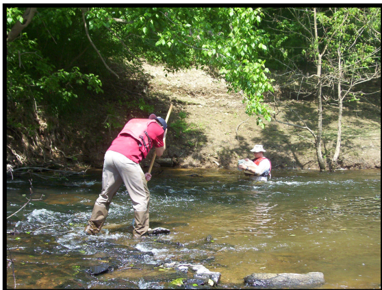
Photos 21 and 22. Sweep net and rock wash sampling for benthic macroinvertebrates at a reference station Source: EcoScience Corporation 2005
