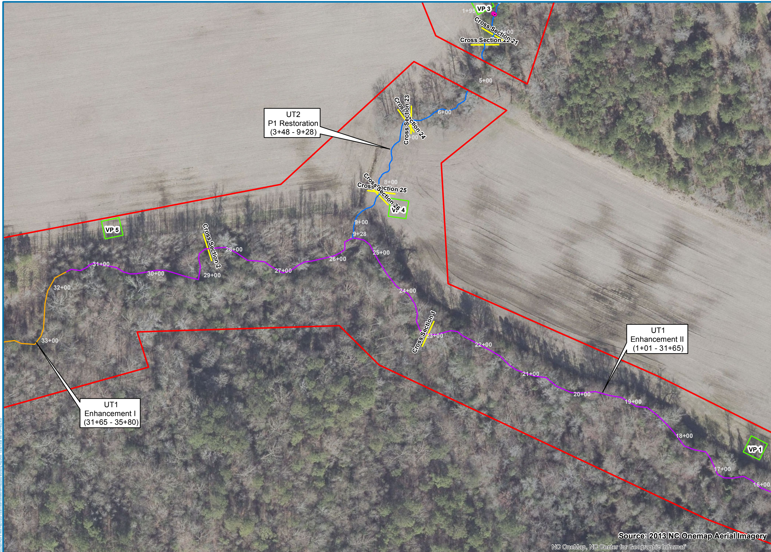
Figure 2b. Cedar Creek Restoration Project UT1 Current Conditions Plan View Map
