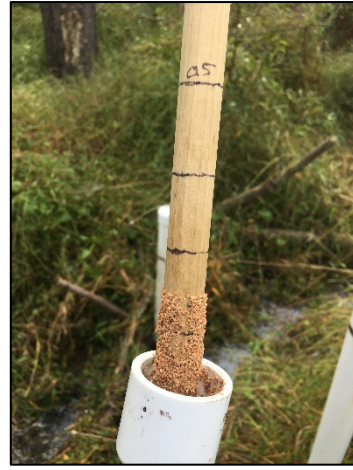
Crest Gauge 3 Reading 0.25 ft (9/15/2018)
