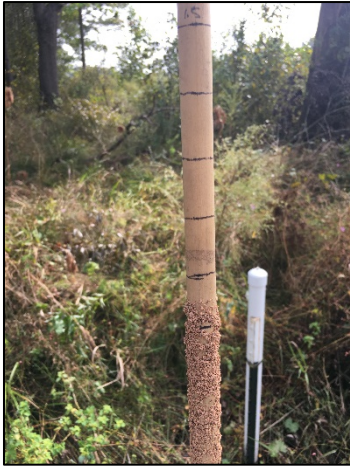
Crest Gauge 1 Reading 1.05 ft (9/15/2018)
