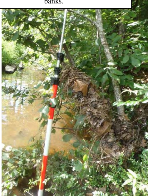
Bankfull Photo 2: Evidence of overbank including wrack and debris in trees and on banks.
