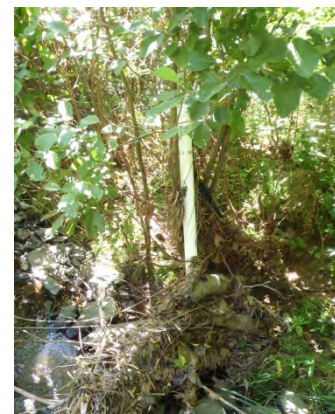
Bankfull Photo 3: Evidence of overbank including wrack and debris on crest gage.
