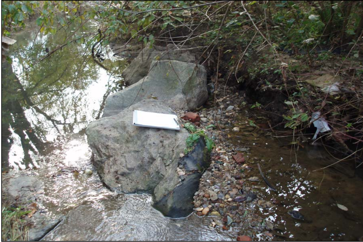
SP7 – Back arm scour on cross vane. Photo taken near Station 14+00. 11/12/07 - MY 04
