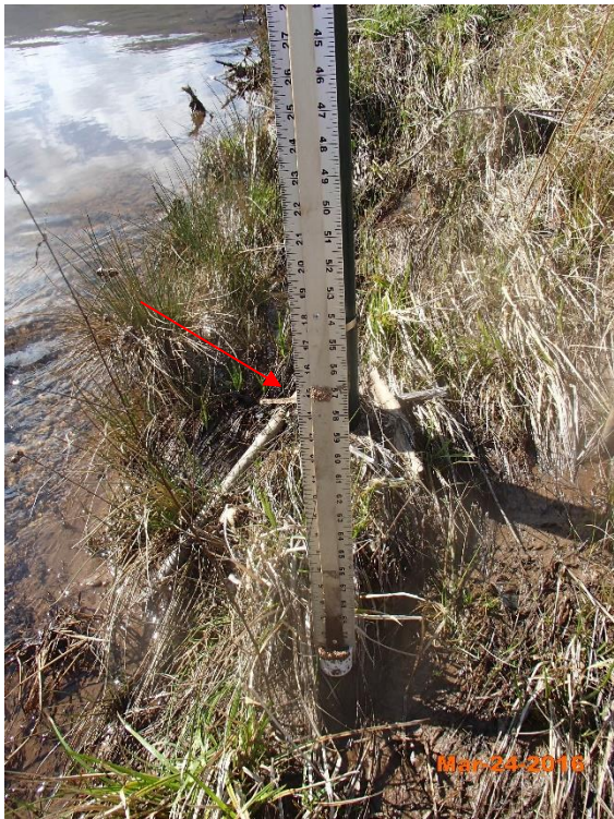
Photo #1 - Cochran Branch Crest Gauge
