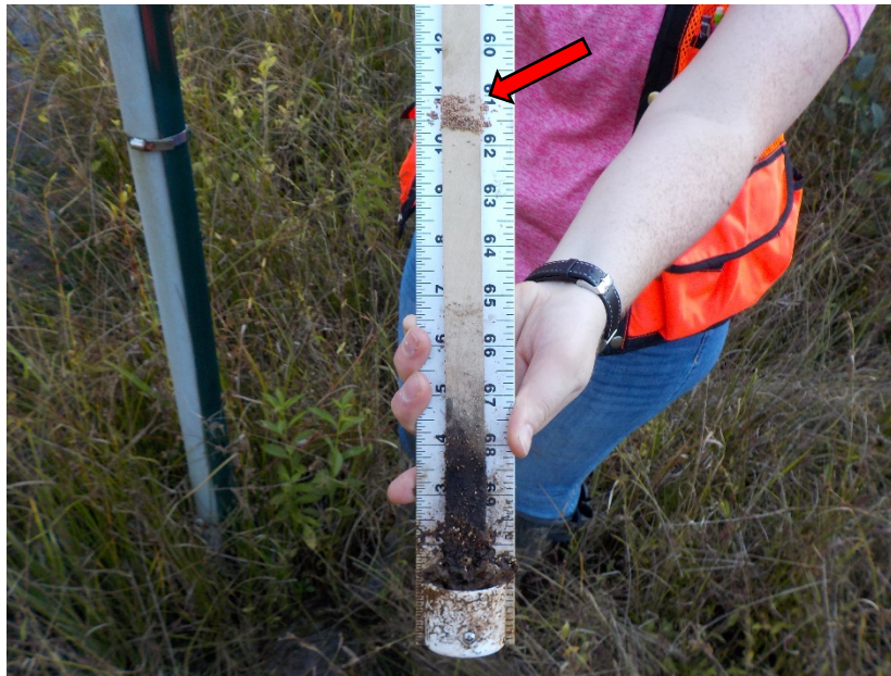
Crest Gauge @ Cochran Branch – 0.92 ft.
