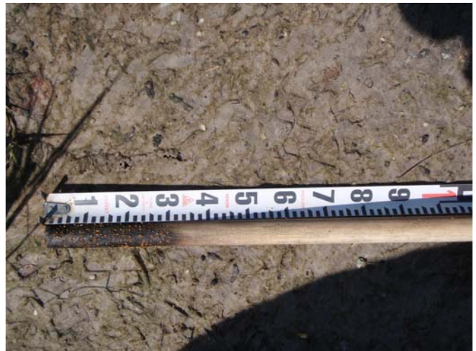
Crest gauge reading of 0.33 feet
