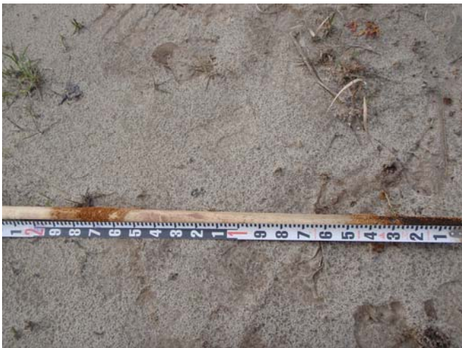
Crest gauge reading of 1.91 feet
