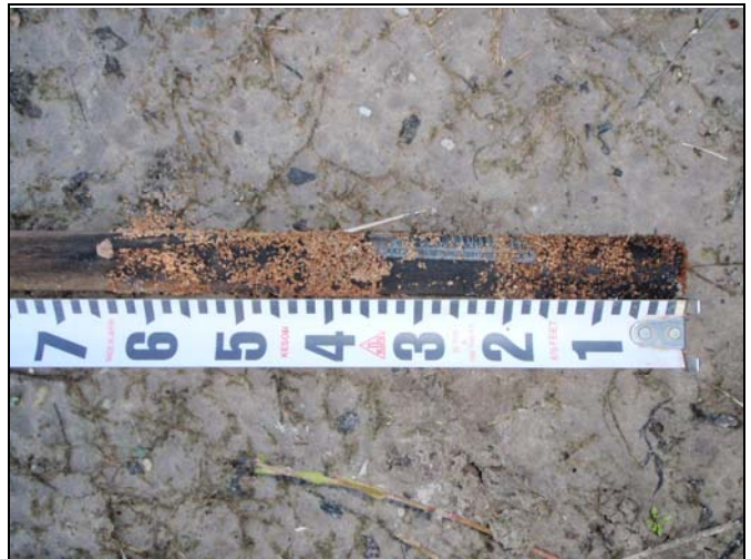
Crest Gauge after Bankfull – 0.63 feet
