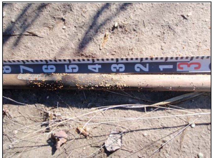
Crest Gauge after Bankfull - 3.72 feet
