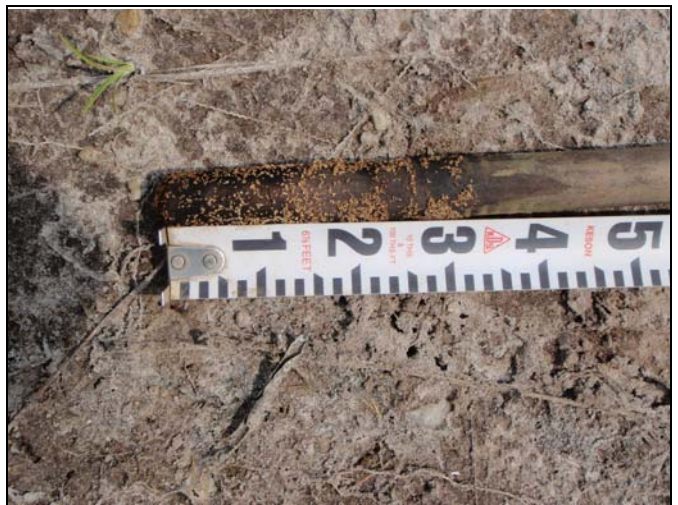
Crest Gauge after Bankfull – 0.31 feet. Bankfull event occurred on or about May 14, 2011
