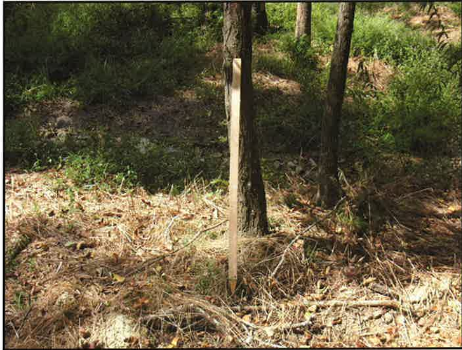
BF 1 Crest Gage on the mainstem of Davis Branch. (EMH&T, Inc. 9/20/09)
