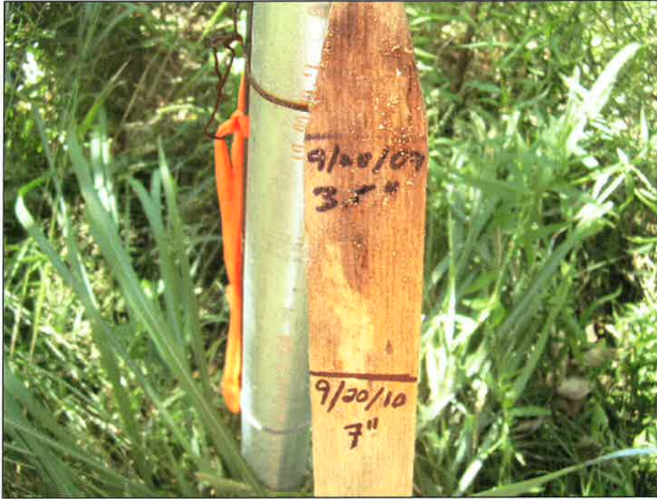
BF 1 Crest Gage on the mainstem of Davis Branch. (EMH&T, Inc. 9/20/10)
